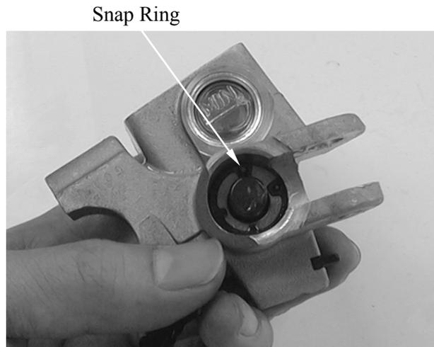
Remove the washer, main piston and spring from the brake master cylinder.
