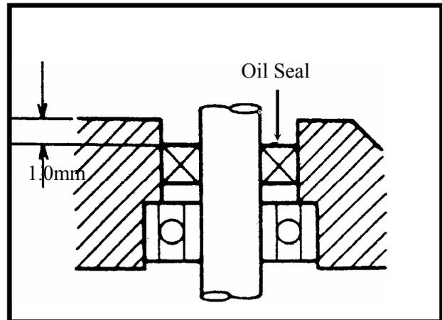
Drive a new crankshaft bearing into the left crankcase.
