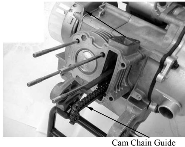
Remove the cylinder gasket and dowel pins. Clean any gasket material from the cylinder surface.
