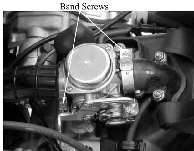
Connect the throttle cable to the carburetor.
