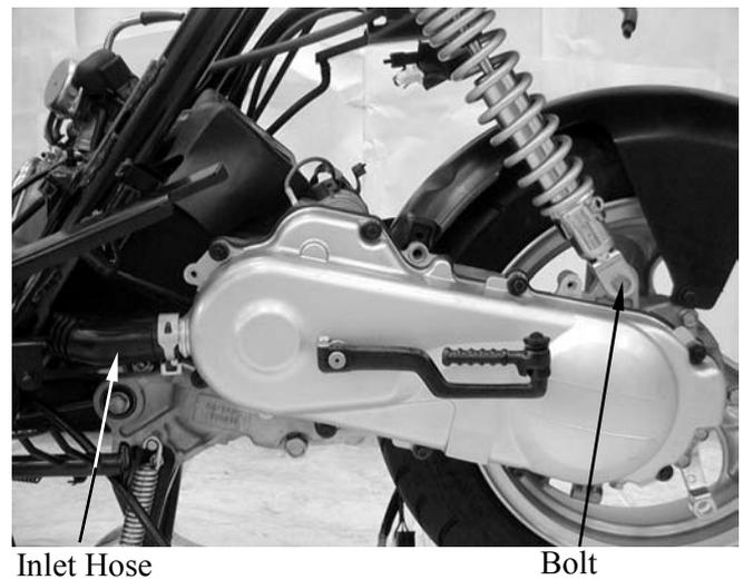
Remove the right and left engine mounting nuts.
