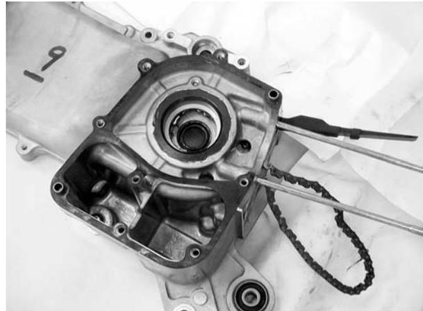
Install the crankshaft into the left crankcase.
