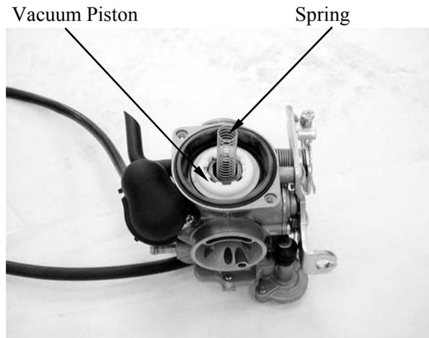
Remove the needle holder, spring and jet needle from the piston.
