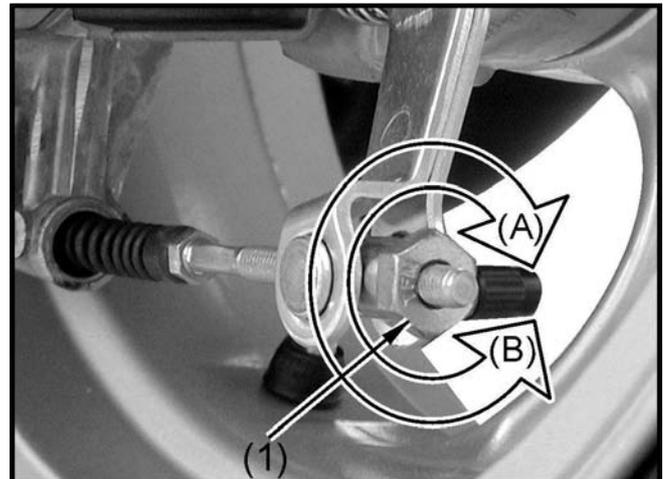
□ Make sure the cut-out on the adjusting nut (2) is seated on the brake arm pin (1) after making final free play adjustment.
