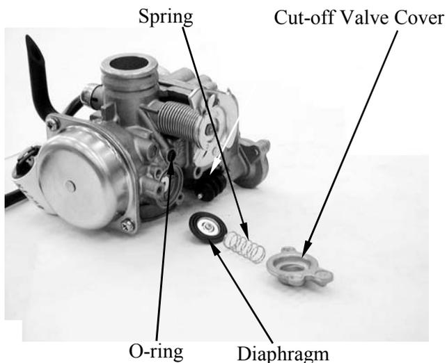
Install and tighten the two screws attaching the air cut-off valve cover.
