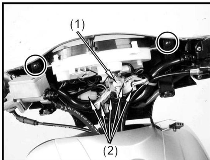
Remove the three screws from the instrument
