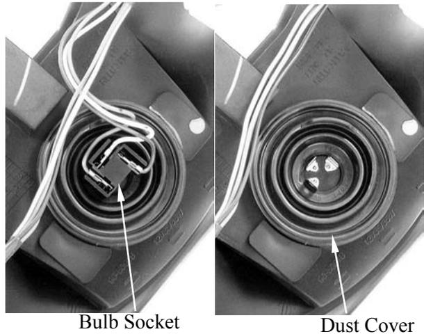
Remove the bulb while pressing down on the pin.
