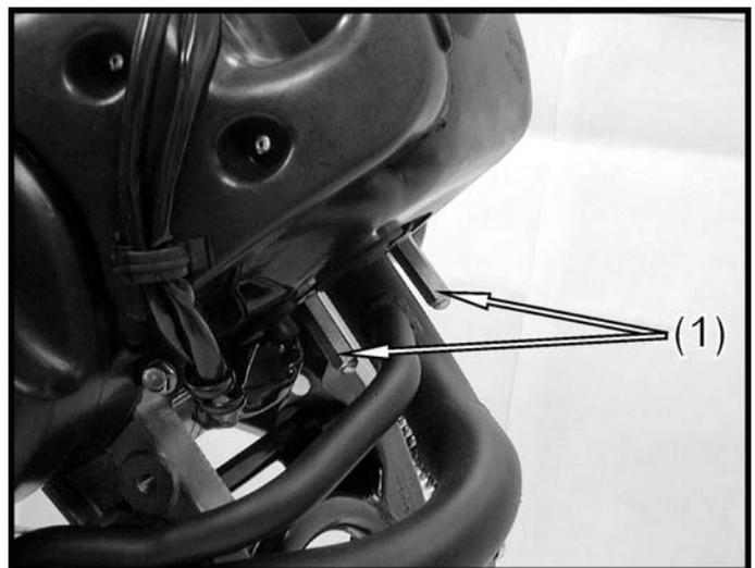
Remove the bolt from the rear lower fender and
