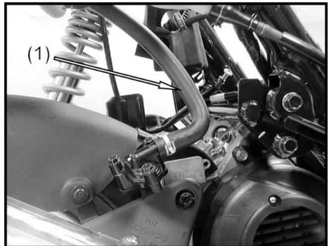
Remove the right and left engine mounting nuts (1).
