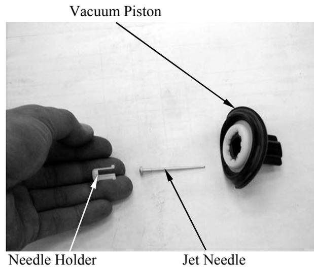
Install the vacuum piston into the carburetor body.
