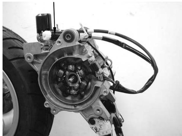
Remove the two pulser coil bolts and pulser coil from the right crankcase.
