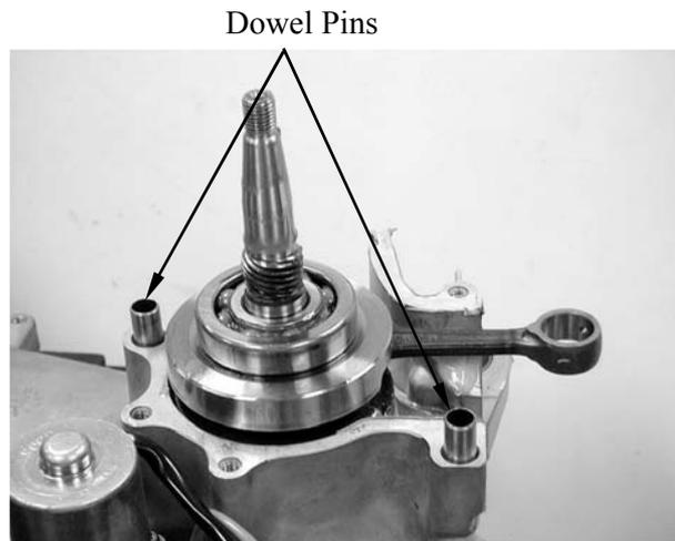
Assemble the crankcase halves.
