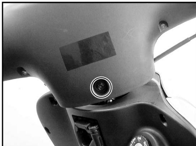
Remove the two mounting screws and disconnect speedometer cable (1).
