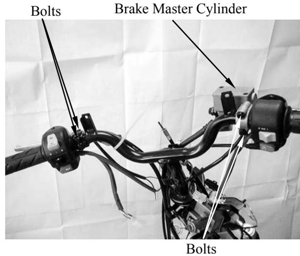
Remove the two right handlebar switch housing bolts and separate the housing.
