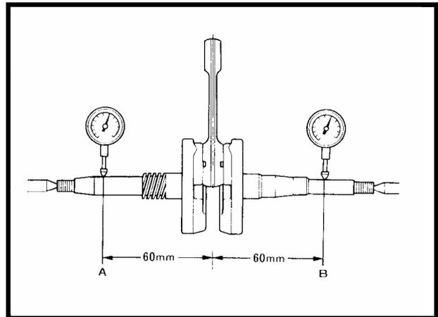
Check the crankshaft bearings for excessive play. The bearings must be replaced if they are noisy or have excessive play.
