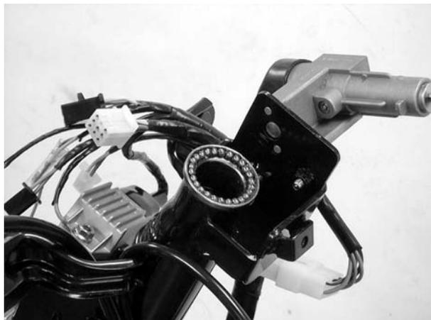
Apply grease to the top cone race and install it.
