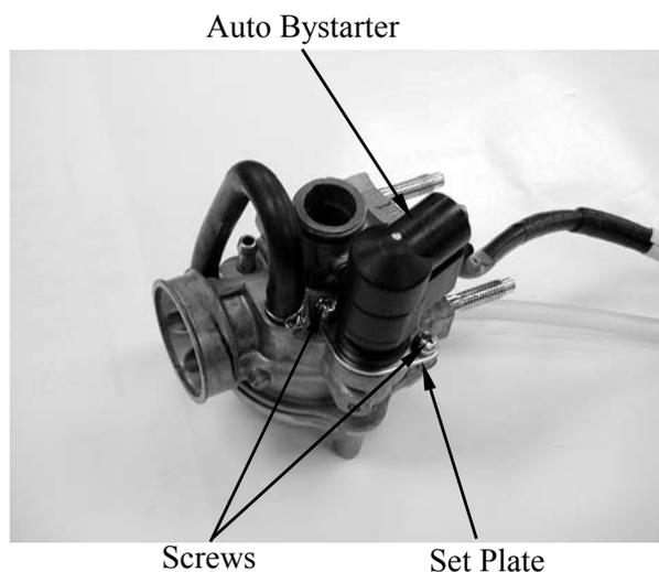
Check the auto bystarter valve and needle for wear or damage.
