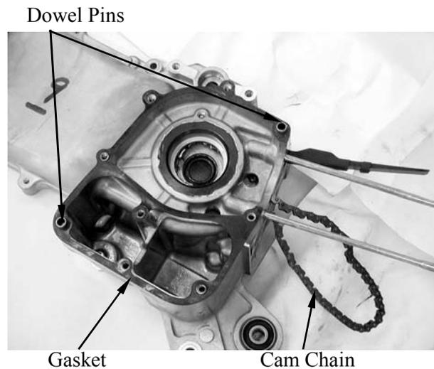
Clean off all gasket material from the crankcase mating surfaces.
