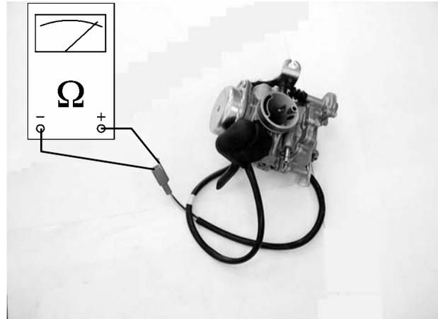
Connect a hose to the fuel enriching circuit of the carburetor. Connect the auto bystarter green/black wire to the positive (+) terminal of a battery and black/white wire to the negative (-) terminal. Wait 5 minutes and blow the hose with mouth. If the passage is blocked, the auto bystarter is normal. Disconnect the auto bystarter from the battery. Wait 30 minutes and blow the hose with mouth. If air can be blown into the hose, the auto bystarter is normal.
