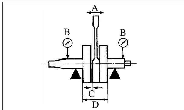
Turn the crankshaft bearings and check for excessive play.
