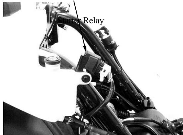
Connect the starter relay green/yellow terminal to the 12V battery positive (+) terminal and the relay yellow/red terminal to the battery negative (-) terminal. Check for continuity between the starter relay red and red/white terminals. The relay is normal if there is continuity.
