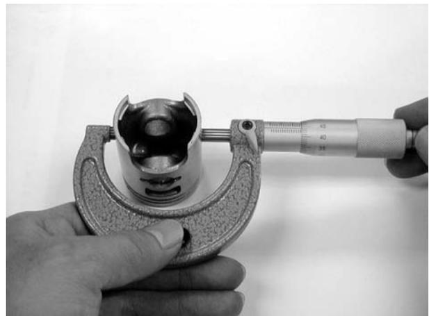
Measure the piston-to-cylinder clearance.
