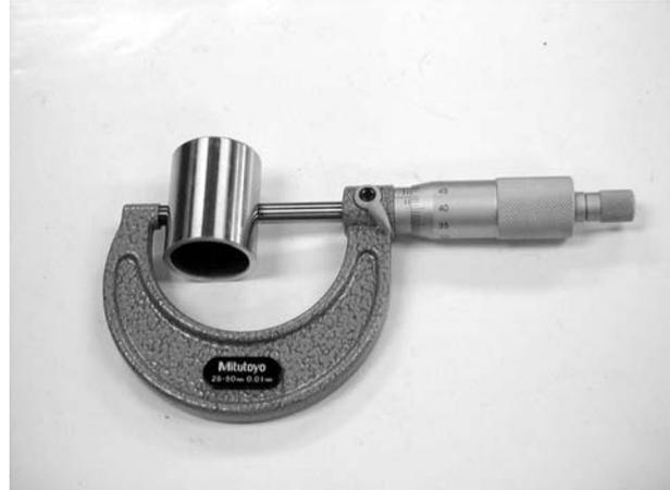
Check the caliper cylinder for scratch or wear and measure the cylinder bore.
