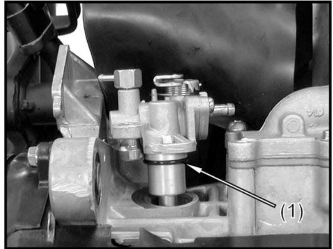
Install the oil pump into the crankcase.
