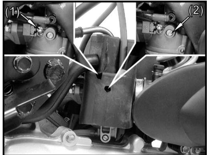
Adjust the idle speed to the specified range by turning the throttle stop screw and pilot screw.
