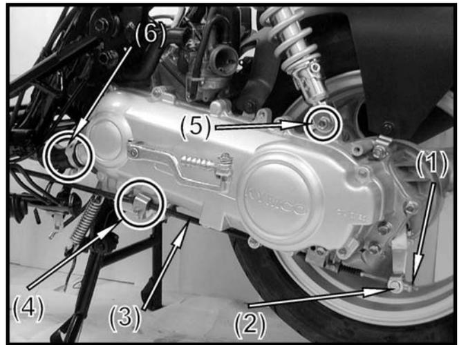
Remove the secondary air hose band (1) from the exhaust muffler and disconnect the secondary air hose.
