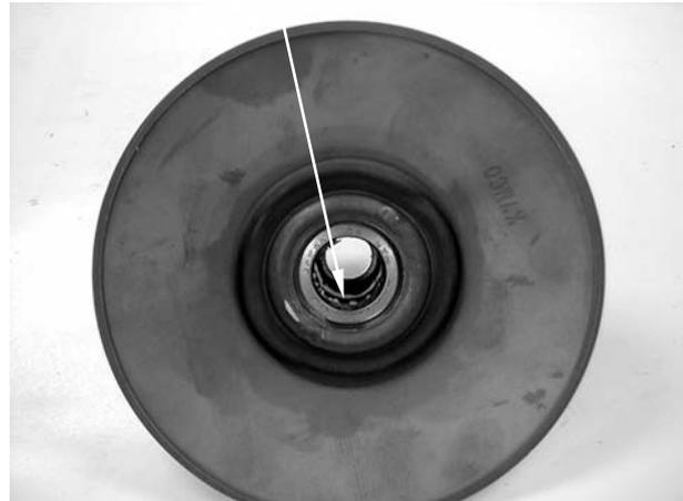
Remove the snap ring and drive the outer bearing out of the driven face.
