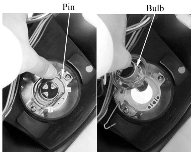
Install a new bulb in the reverse order of removal.
