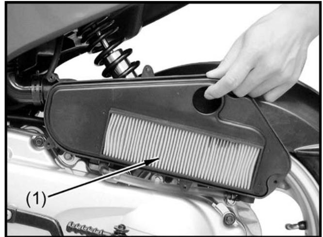
3. Clean the air cleaner element with compressed air.
