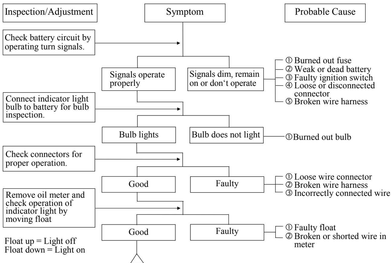
2. Motor oil is sufficient but the indicator light remains on (Ignition switch ON)
