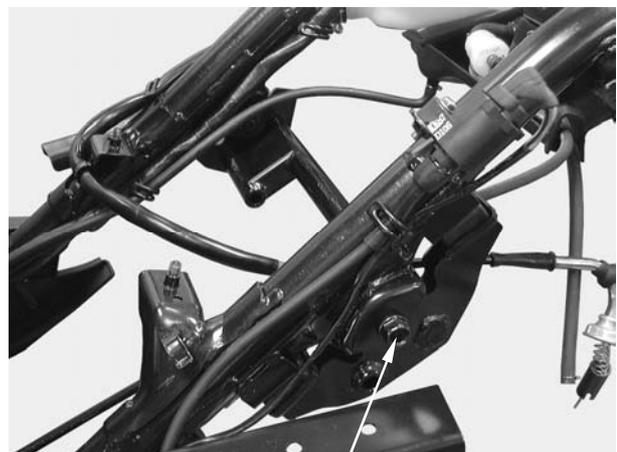
Engine Hanger Bracket Bolt
