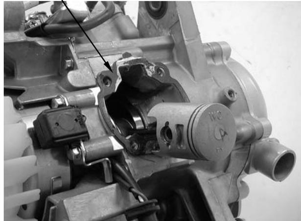
Make sure that the ring end gaps are aligned with the piston ring pins in the ring grooves.
