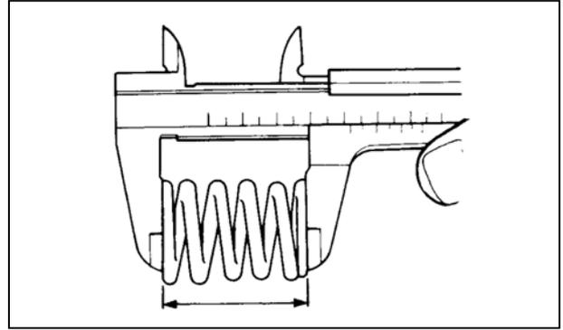
Measure compressed force (valve spring) and installed length.
