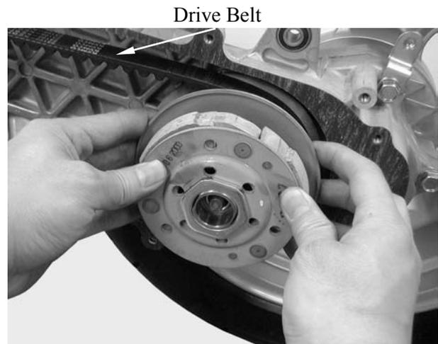
Set the drive belt on the drive pulley.
