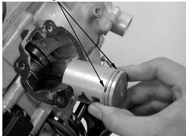
Lubricate the cylinder inside and piston rings with engine oil and install the piston into the cylinder while compressing the piston rings.
