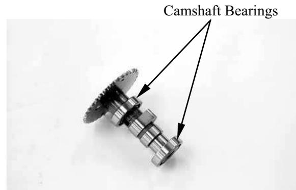
Inspect camshaft lobes for pitting/scratches/blue discoloration.
