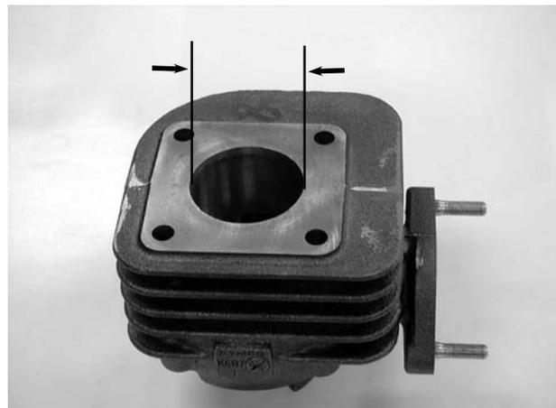
Inspect the top of the cylinder for warpage.
