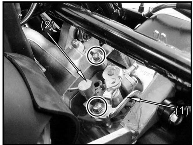
Connect the oil inlet line (1) and oil outlet
