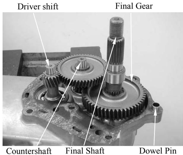
Countershaft Final Shaft Dowel Pin
