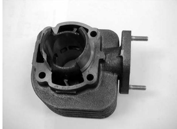
Measure the cylinder bore at three levels of A, B and C in both X and Y directions. Avoid the port area. Take the maximum figure measured to determine the cylinder bore.
