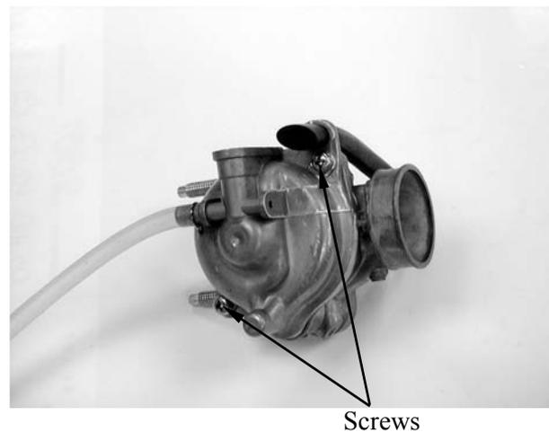
Remove the screw and O-ring.
