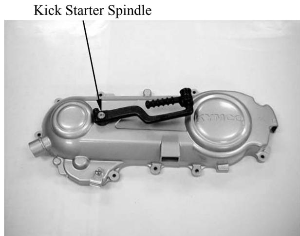
Slightly rotate the kick starter spindle to remove the kick starter driven gear together with the friction spring.
