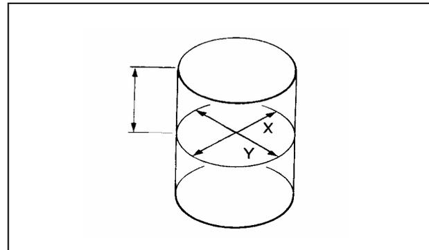
The true roundness is the difference between the values measured in X and Y directions. The cylindricity (difference between the values measured at the three levels) is subject to the maximum value calculated.
