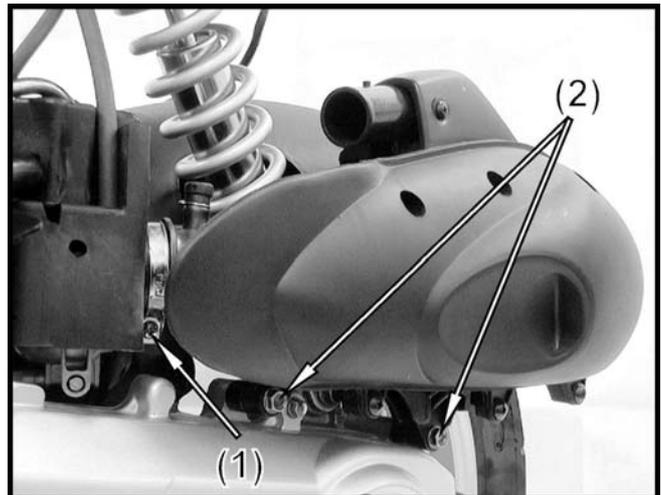
Slide the rubber sleeve up to expose the carburetor.
