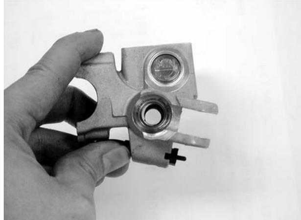
Measure the brake master cylinder piston O.D.
