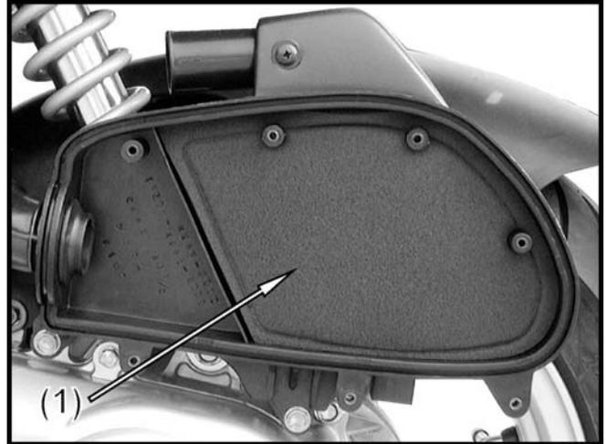
Wash the air cleaner element in detergent oil, squeeze out and allow to dry.
