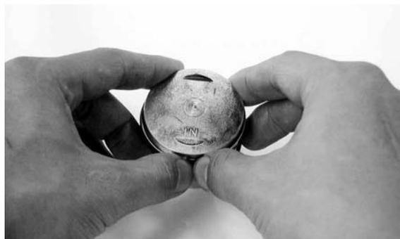
Inspect the piston wall for wear/scratches/damage.
