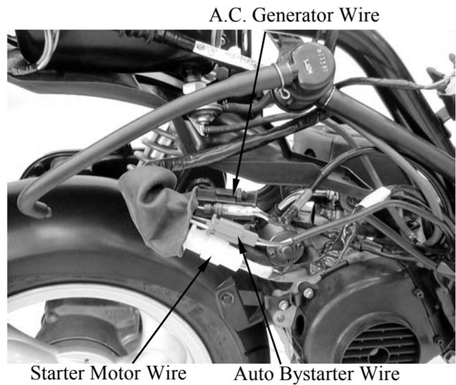
Remove the spark plug cap.
