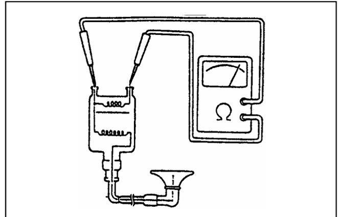
Measure the secondary coil resistance between the spark plug cap and the primary coil terminal as Figure A shown.
