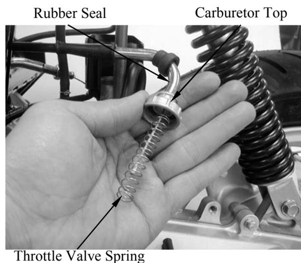
Connect the throttle cable to the throttle valve.
