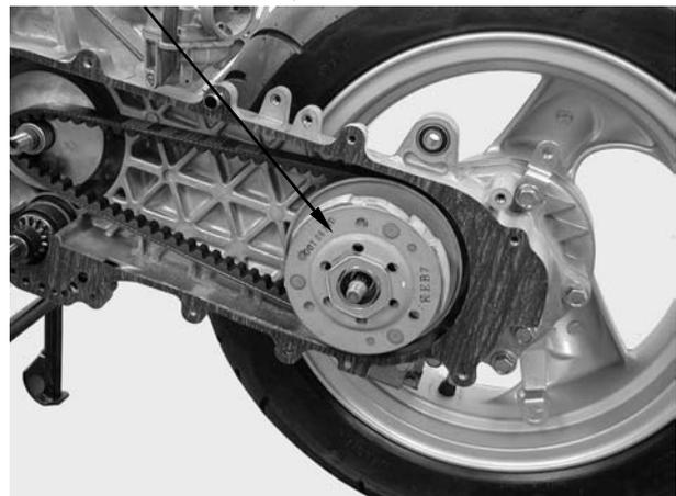
Install the clutch outer. Hold the clutch outer with the universal holder. Install and tighten the 14mm clutch outer nut.
