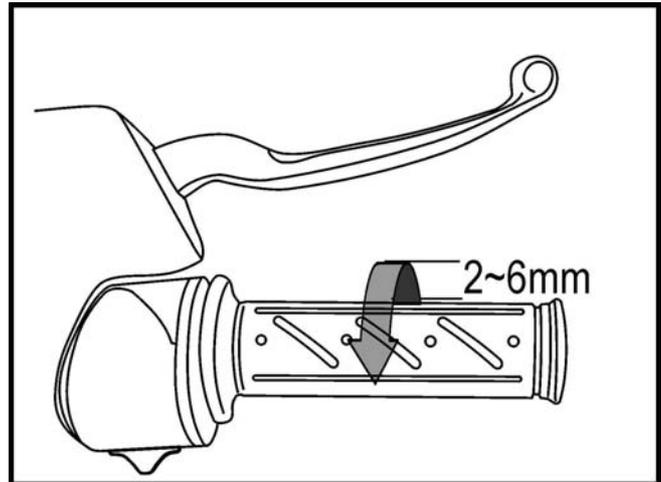
If the throttle grip free play does not fall within the specified range, adjust by loosening the lock nut (1) and turning the adjusting nut (2).
