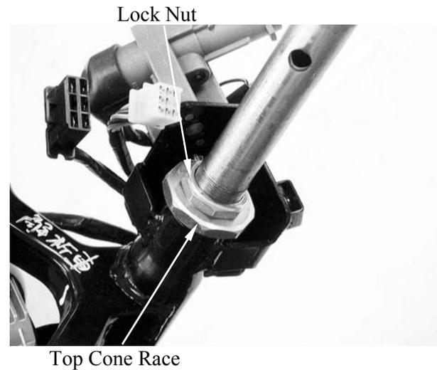
Remove steering stem lock nut with lock the lock nut socket wrench.
