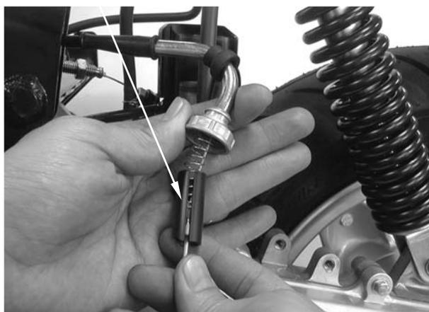
Remove the throttle valve spring, carburetor top and rubber seal.
