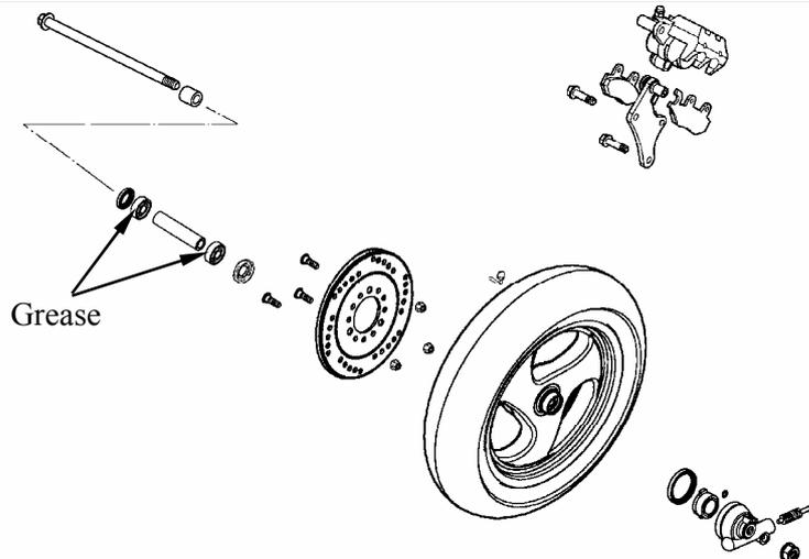
Pack all bearing cavities with grease.
