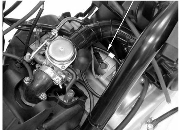
Disconnect the fuel tube from carburetor.
