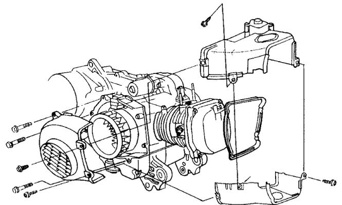
Remove seal shroud, then remove two bolts and cylinder head.
