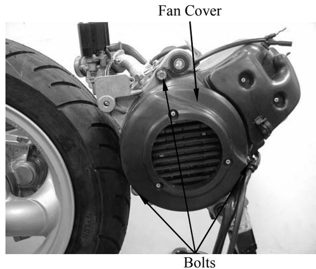
Remove the cooling fan by removing the four bolts.
