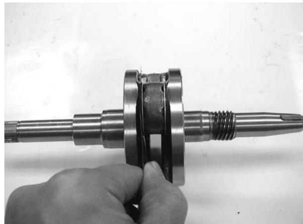
Measure the connecting rod big end radial clearance at two points in the X and Y directions.
