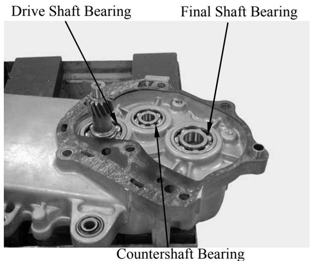
Inspect the drive shaft and gear for wear or damage.
