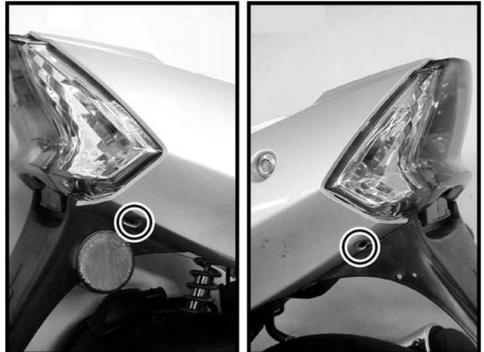
Remove the two screws from the rear body cover.
