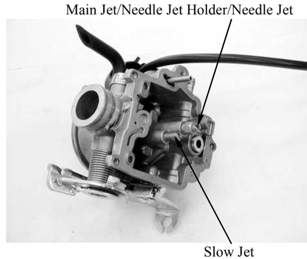
Clean the removed the main jet, needle jet holder, needle jet and slow jet with detergent oil.
